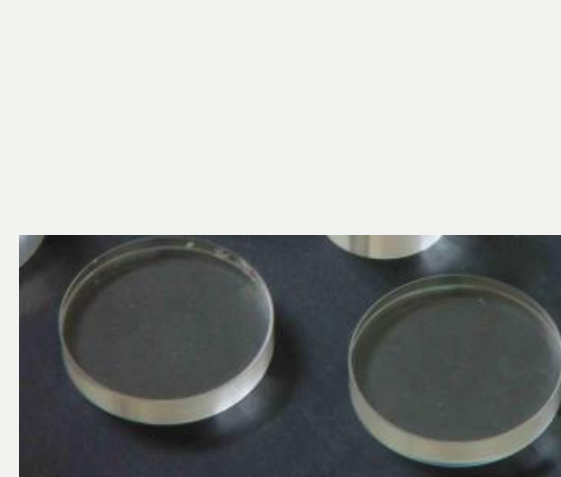
Figure 2: Cesium Bromide archetype Crystals used to absorb X-Rays
